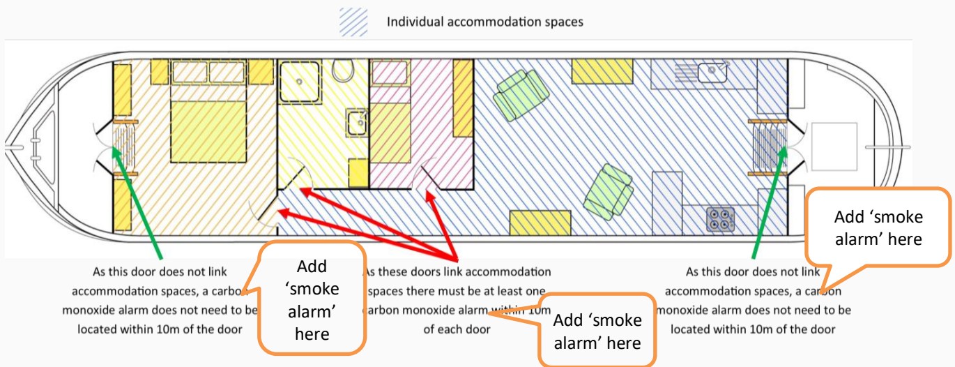
Fig 1. To be compliant at Checks 6.4.1 and 6.5.2, CO and smoke alarms must be located within 10m of the three doors that link accommodation spaces.
