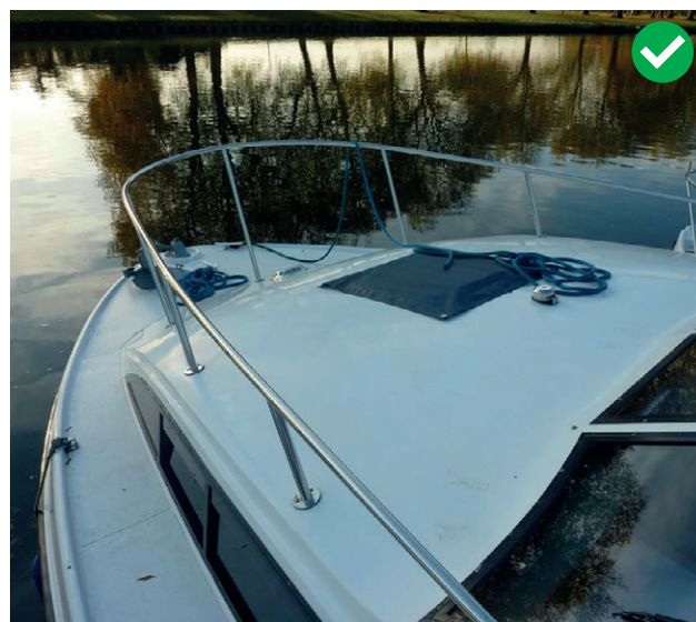
Fig 1 – two different types of pulpit, both of which provide suitable protection to the otherwise exposed bow deck and would therefore be BSS compliant with Check 10.1.2. Hire operators are encouraged to install pulpits wherever practical.
