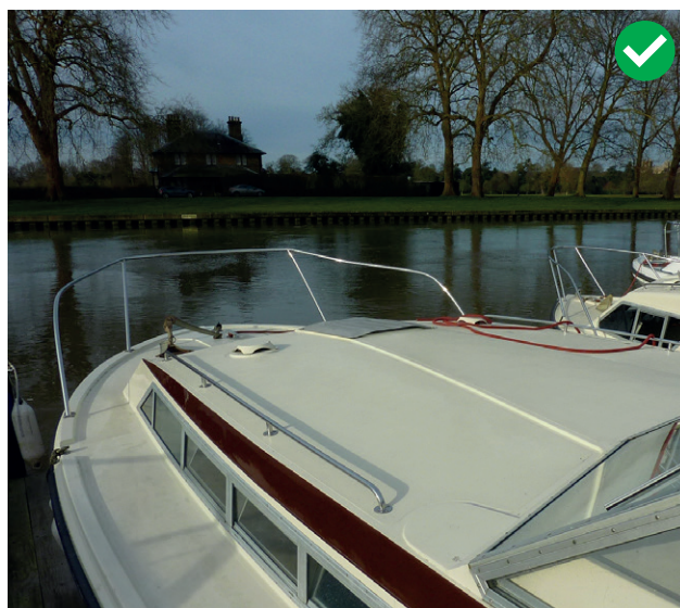
Fig 1 – two different types of pulpit, both of which provide suitable protection to the otherwise exposed bow deck and would therefore be BSS compliant with Check 10.1.2. Hire operators are encouraged to install pulpits wherever practical.
