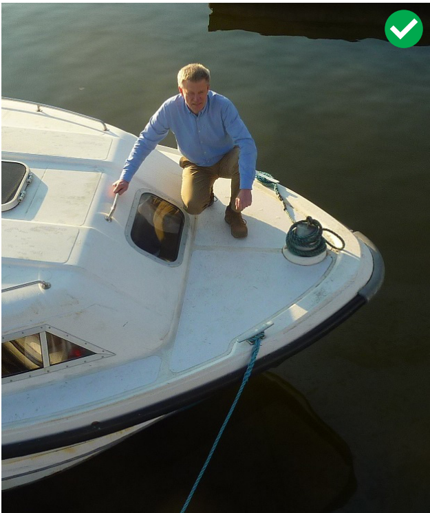
Fig 6 – The hire operator of this cruiser (as seen previously at Fig 3) has chosen to add a handhold to the cabin structure above the forward window. This arrangement is now compliant at Check 10.1.2 as the hirer can reach a suitable handhold from anywhere on the forward deck and the gap between the handholds is less than 1.5m.
