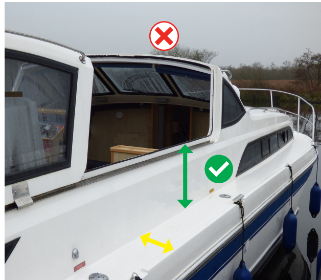
Fig 12. In this example the gap between the cabin roof handrails is greater than 1.5m and is therefore not compliant. However, even though the side deck is less than 300mm wide, the top of the coaming (which the hire operator has designated as a handhold) is greater than 350mm above the side deck, which is compliant.
