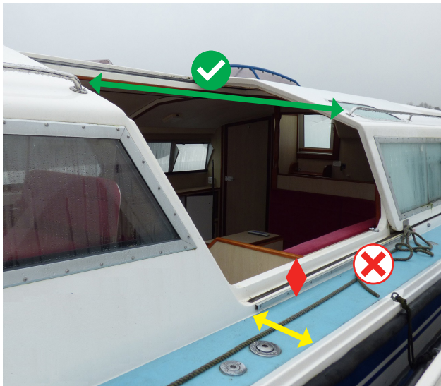
Fig 11. In this example the gap between the cabin roof handrails is less than 1.5m, which is compliant. The coaming cannot be considered as a handhold because the side deck is less than 300mm wide and the coaming is less than 350mm above the side deck.
