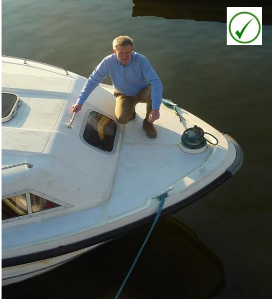
Fig 6 – The hire operator of this cruiser (as seen previously at Fig 3) has chosen to add a handhold to the cabin structure above the forward window. This arrangement is now compliant at Check 10.1.2 as the hirer can reach a suitable handhold from anywhere on the forward deck and the gap between the handholds is less than 1.5m.
