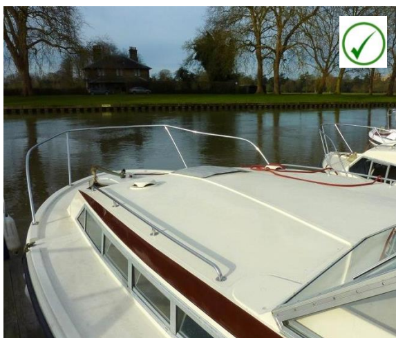
Fig 1 – two different types of pulpit, both of which provide suitable protection to the otherwise exposed bow deck and would therefore be BSS compliant with Check 10.1.2. Hire operators are encouraged to install pulpits wherever practical.
