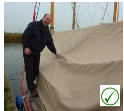
Fig 13 – cabin roof handrail accessible through the tent canvas.
