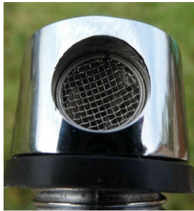
Proprietary flame arrest with a mesh of exactly 11 wires/cm
