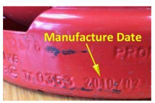
At the very bottom of the base ring the third row of text shows the date of manufacture i.e. 2008, 2009, 2010 or 2011.
