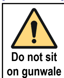
Do not sit or stand on the gunwale (using ISO 7010 – W001 “General warning”)
