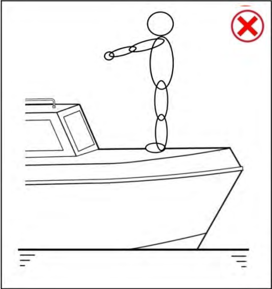
Fig 2 – bow deck on cruiser is not compliant with Check 10.1.2 as there is no handhold available. Even if the hirer were to crouch down there would be no suitable handholds on the forward deck.
