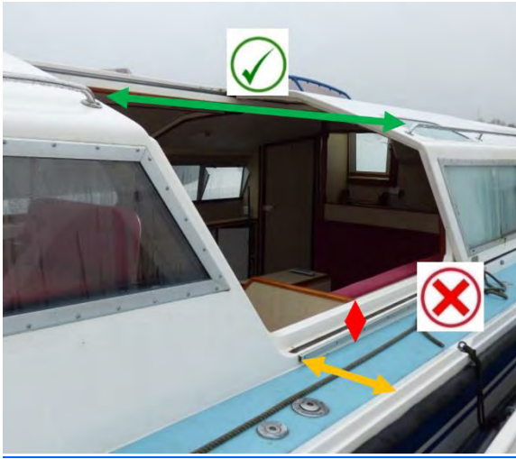
Fig 11. In this example the gap between the cabin roof handrails is less than 1.5m, which is compliant. The coaming cannot be considered as a handhold because the side deck is less than 300mm wide and the coaming is less than 350mm above the side deck.
