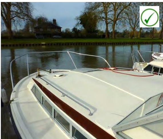
Fig 1 – two different types of pulpits, both of which provide suitable protection to the otherwise exposed bow deck and would therefore be BSS compliant with Check 10.1.2. Hire operators are encouraged to install pulpits wherever practical.
