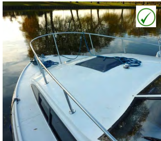
Fig 1 – two different types of pulpits, both of which provide suitable protection to the otherwise exposed bow deck and would therefore be BSS compliant with Check 10.1.2. Hire operators are encouraged to install pulpits wherever practical.
